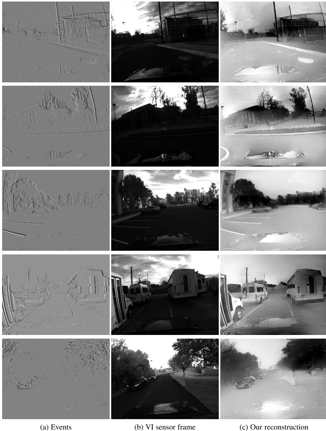
Fig. 21. Example HDR reconstructions on the MVSEC automotive dataset [43]. The standard frames were recorded with a high-quality VI sensor with auto-exposure activated. Because the camera is facing directly the sun, the standard frames (b) are either under- or over-exposed since the limited dynamic range of the standard sensor cannot cope with the high dynamic range of the scene. By contrast, the events (a) capture the whole dynamic range of the scene, which our method successfully reconstructs to high dynamic range images (c), allow to discover details that were not visible in the standard frames.
