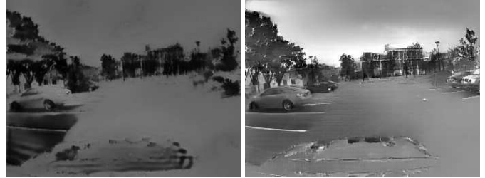
Fig. 17. Reconstruction from (i) a network trained only on real event data from the DAVIS240C sensor (left), and (ii) a network trained only on simulated event data (right). This sequence is from the MVSEC dataset, and was recorded with a mDAVIS346 sensor.
